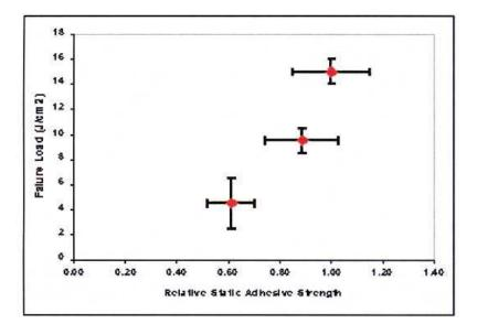
Figure 2. Comparison of LBI failure fluence with tensile tests for variable adhesive quality.
