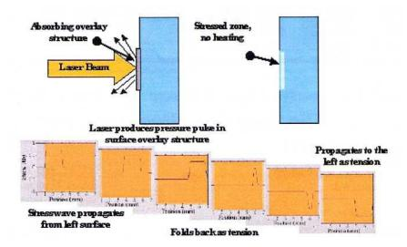
Figure 1. One-dimensional approximation for laser based shockwave generation and stress pulse propagation in a solid slab.
