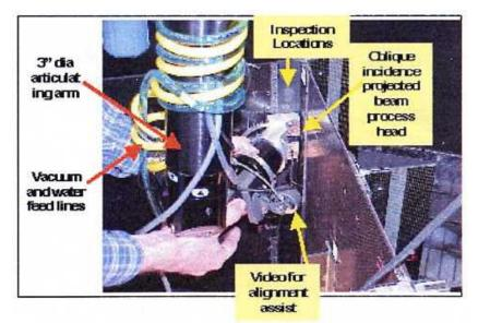
Figure 4. Beam delivery system with process head for use in an assembly environment.
