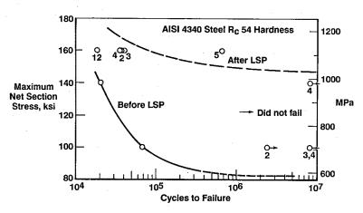
Figure 8 Fatigue improvement in 4340 steel after laser shock processing.
