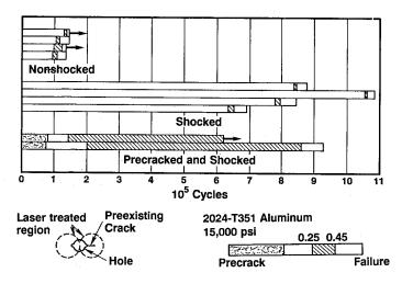
Figure 7 Laser shock processing increases the fatigue life of precracked specimens. Left = laser shock process pattern. Right = fatigue life.
