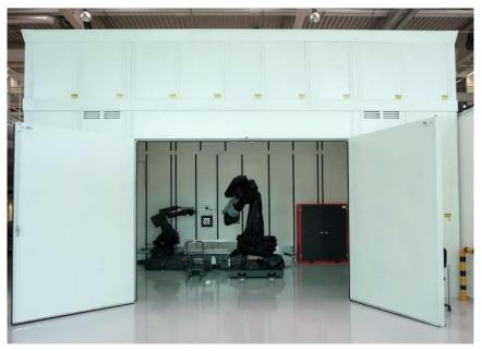
The massive new laser peening cell at the ZAL TechCenter
